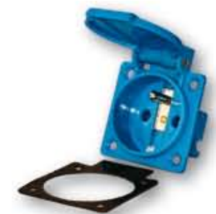
MAINS OUTLET SOCKET Order Code: 1150 230Vac/ 16A outlet socket with Belgian/French grounding. (IP54) Dimensions= 50x50mm
